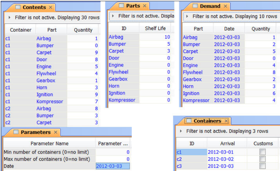
Figure 2-2 Input data tables of the ContainerYard application
